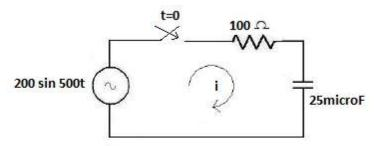
5.In the circuit shown in figure, Find the transient current when the switch is closed at t=0. Assume zero initial conditions.
