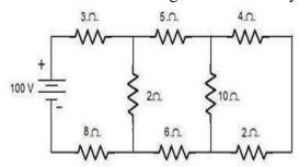
2.Calculate a) the equivalent resistances across the terminals of the supply, b) total current supplied by the source and c) power delivered to 16 ohm resistor in the circuit shown in figure.
